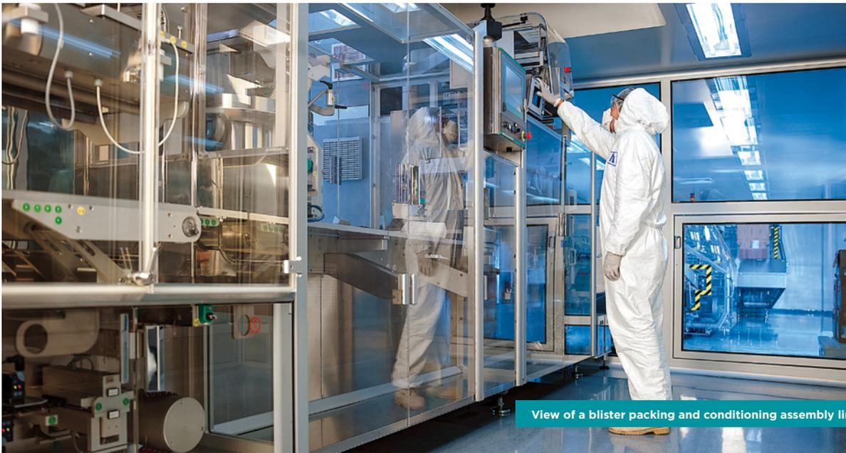
View of a blister packing and conditioning assembly line
